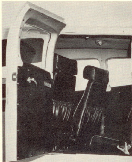
The 1973 Sierra, top of Beech's light single-engine line, has a new entry door on the left side of the fuselage to facilitate entry to and exit from the optional fifth and sixth seats.
